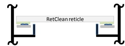
Contamination resting on the surface of the robot arm comes into contact with the poly when the robot lifts the RetClean reticle.
